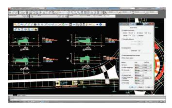
Save time by producing multiple cross sections when checking for potential conflict between terrain elevation and a vehicle's 3D swept path.
