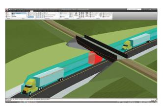
>> Create a 3D vehicle using custom roofline and ground clearance values for the front, rear, and wheelbase of a vehicle.
