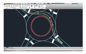
>> Modify end nodes for different positioning and sweep angle for Corner and Oversteer Path
