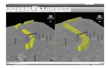
>> Hatch the 3D vehicle swept path to check clearances issues during a vehicle simulation.
