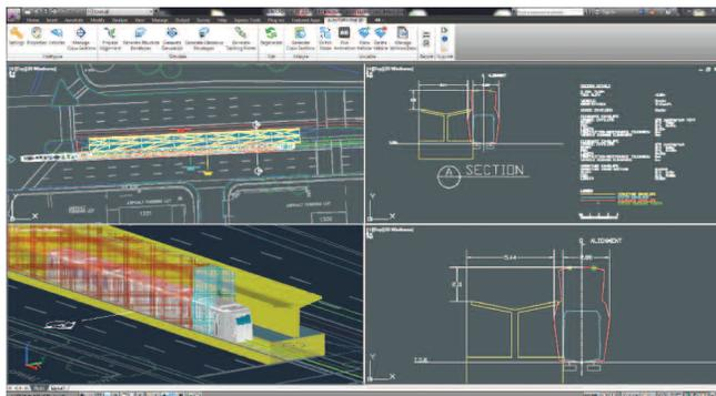
» Accurately scale dimensions off the full scale report vehicle envelope clearance and tracking points relative to any structure envelopes.
