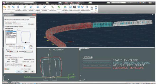
» Save time by making adjustments to the construction-maintenance tolerance and vehicle running clearance envelopes directly in the software.
