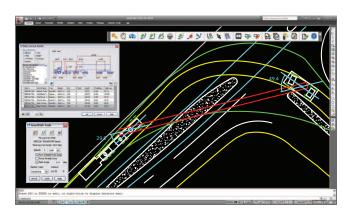
>> Check the drive path of large, complex vehicles carrying cargo to prevent damage to the load or surrounding structures.
