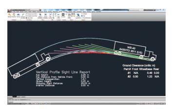
Safety comes first. Check vertical sightlines using driver eye height, object height, interval and sight line distances
